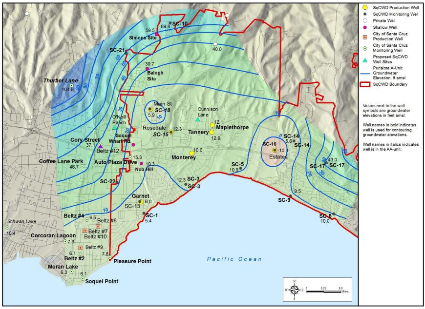
Figure 3-2 (2010): Groundwater Elevation Contours, Purisima A-Unit, Spring 2010
