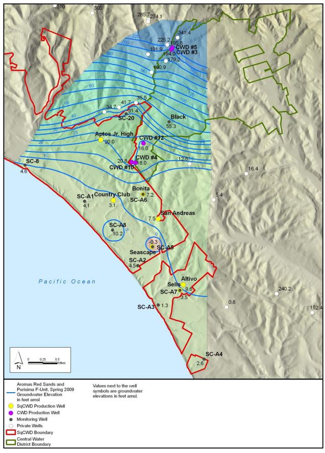
Figure 5-2 (2009): Groundwater Elevation Contours, Aromas Area, Spring 2009
