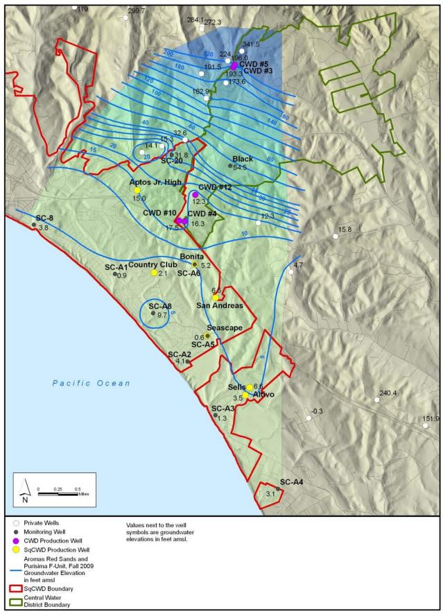
Figure 5-3 (2009): Groundwater Elevation Contours, Aromas Area, Fall 2009
