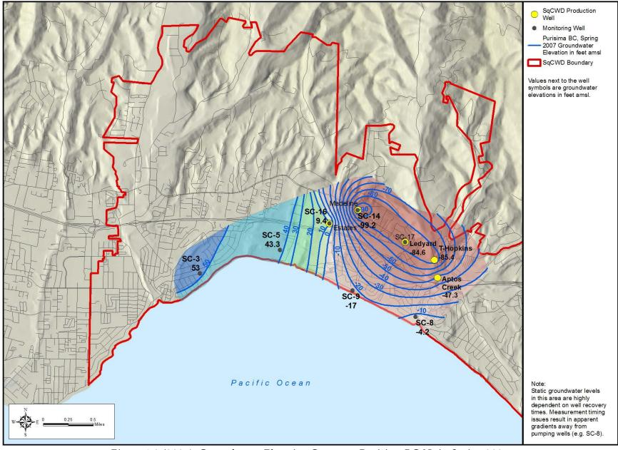
Figure 4-2 (2007): Groundwater Elevation Contours, Purisima BC-Unit, Spring 2007
