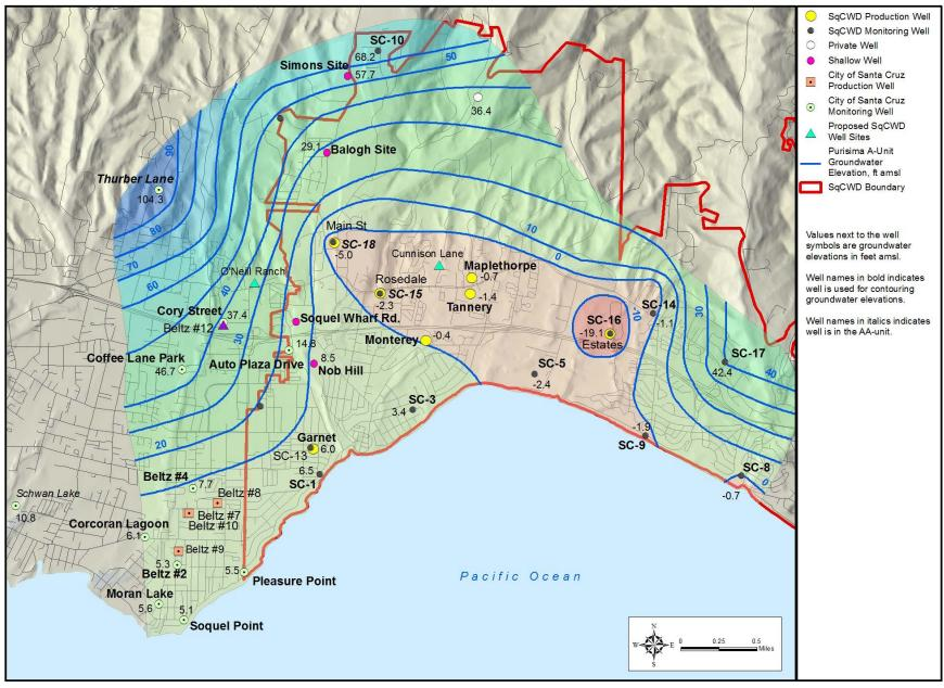
Figure 3-3 (2010): Groundwater Elevation Contours, Purisima A-Unit, Fall 2010
