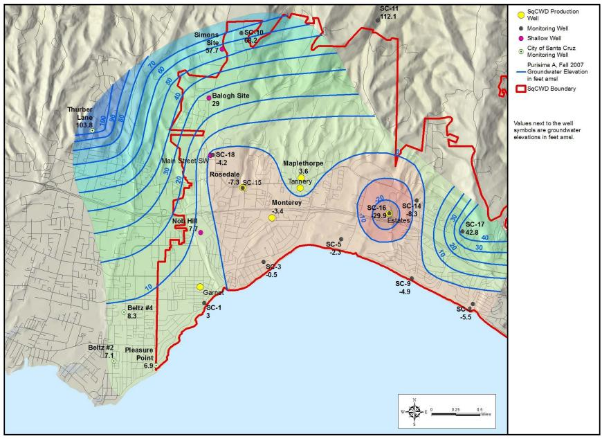
Figure 3-3 (2007): Groundwater Elevation Contours, Purisima A-Unit, Fall 2007
