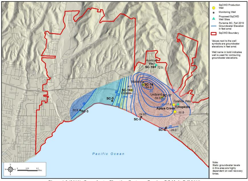
Figure 4-3 (2010): Groundwater Elevation Contours, Pursima BC-Unit, Fall 2010
