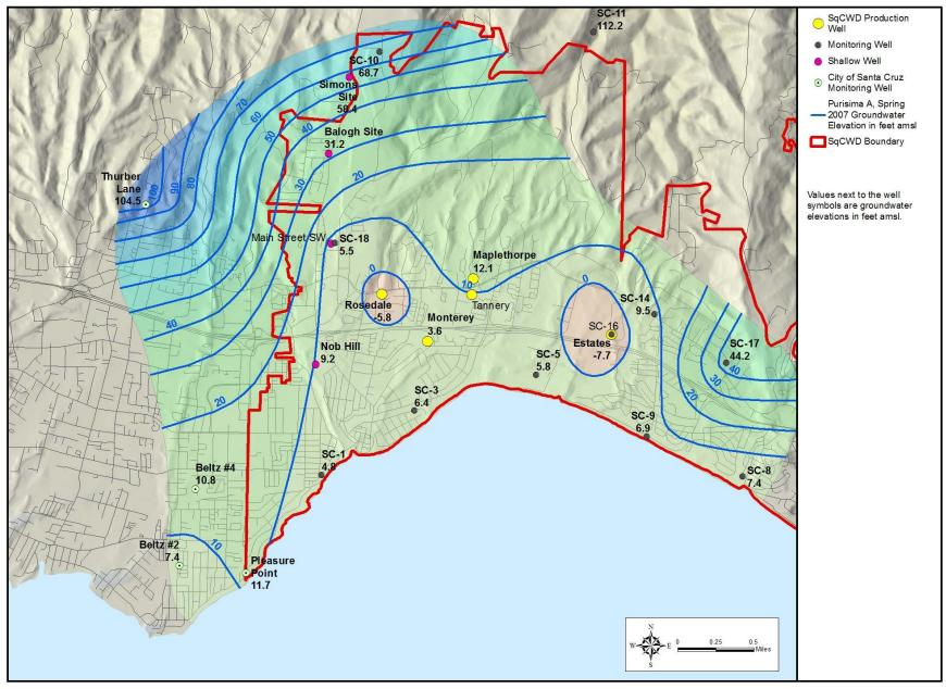
Figure 3-1 (2007): Groundwater Elevation Contours, Purisima A-Unit, Spring 2007
