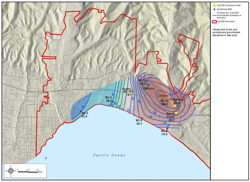
Figure 4-3 (2007): Groundwater Elevation Contours, Purisima BC-Unit, Fall 2007
