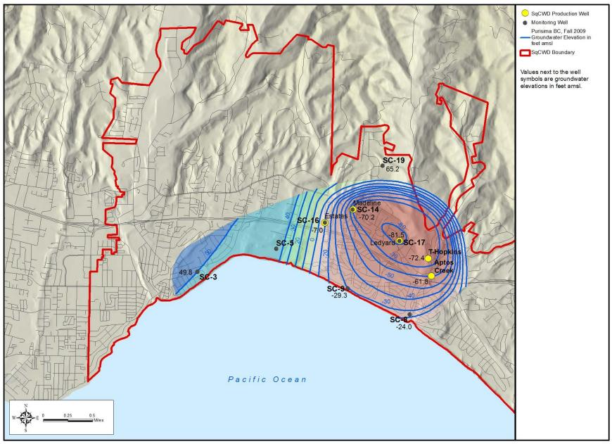
Figure 4-3 (2009): Groundwater Elevation Contours, Pursima BC-Unit, Fall 2009
