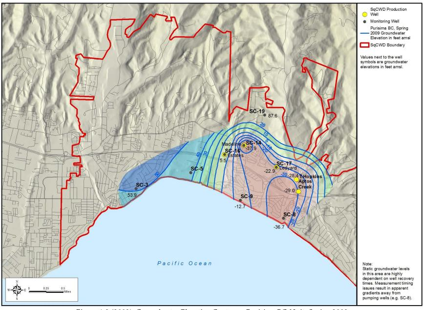
Figure 4-2 (2009): Groundwater Elevation Contours, Purisima BC-Unit, Spring 2009
