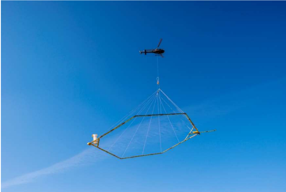
Figure 3 SkyTEM system towed 100 feet below the helicopter. Photo from another survey
