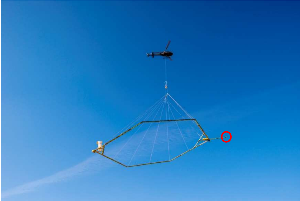
Figure 6 Total Magnetic field sensor mounted in the front of the carrier frame and only measuring in the TDEM off-times.
