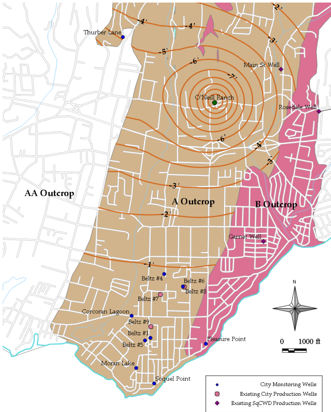
Figure 15. Water Level Changes in A Unit for O'Neill Ranch Well Pumping Using Parameters Matching Main Street Pump Test Data at Wells 18A and 18AA and Assuming No Flow from West of A Unit Outcrop
