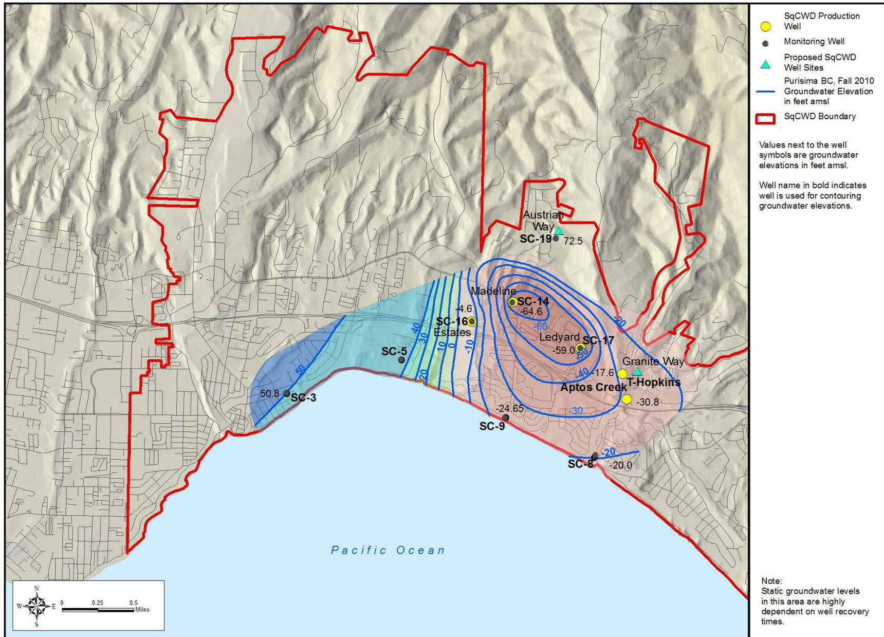
Figure 4-3 (2010): Groundwater Elevation Contours, Purisima BC-Unit, Fall 2010
