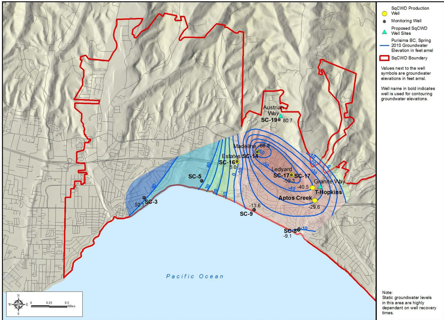
Figure 4-2 (2010): Groundwater Elevation Contours, Purisima BC-Unit, Spring 2010
