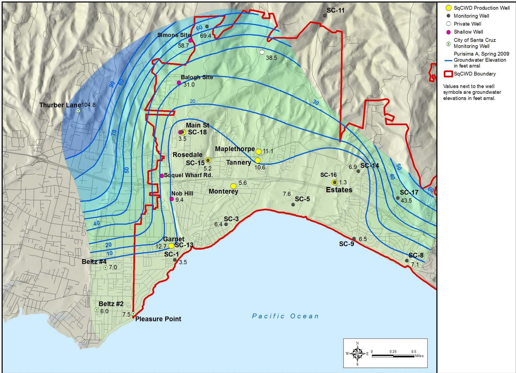
Figure 3-2 (2009): Groundwater Elevation Contours, Purisima A-Unit, Spring 2009
