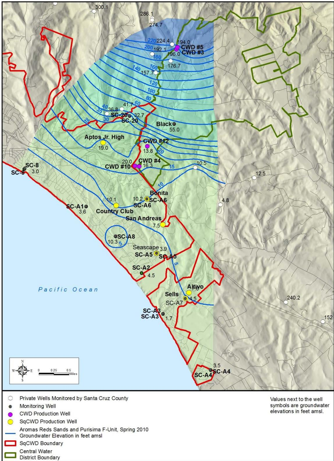
Figure 5-2 (2010): Groundwater Elevation Contours, Aromas Area, Spring 2010
