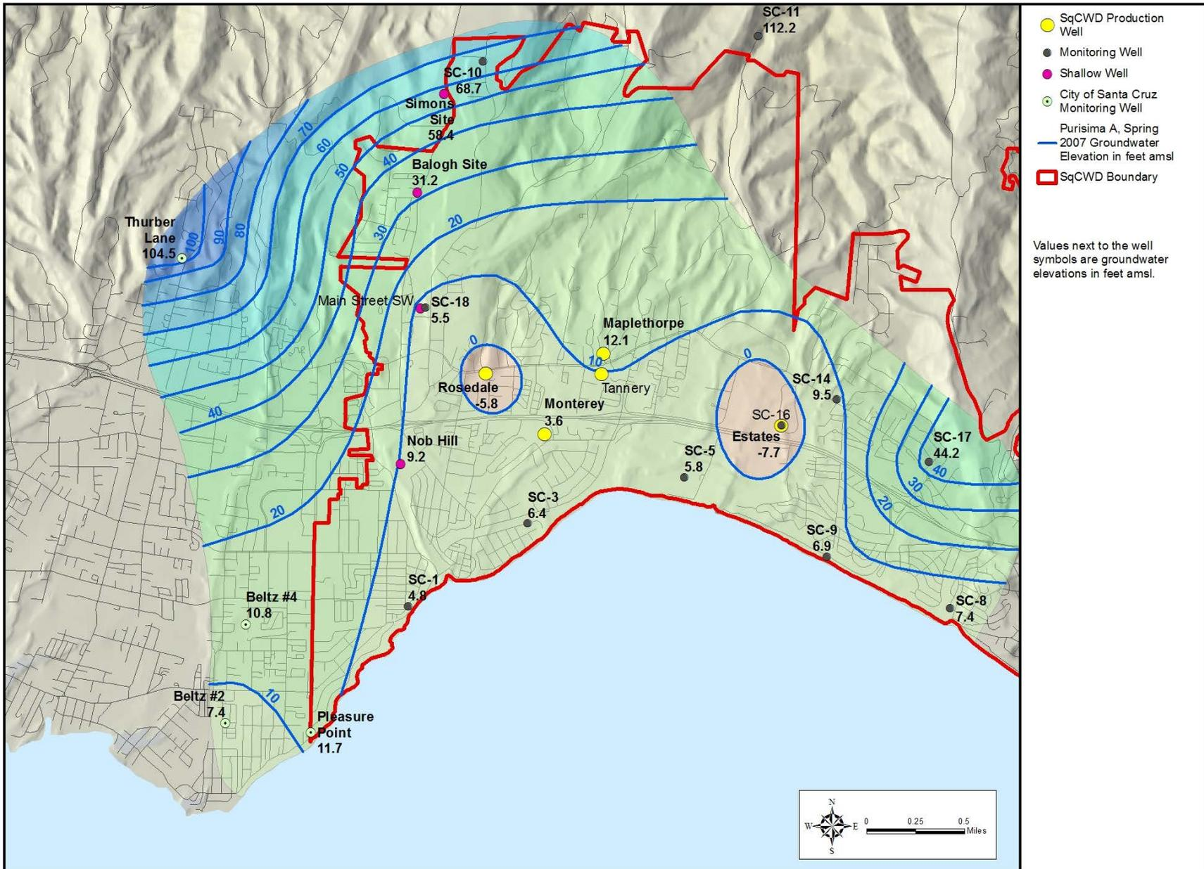
Figure 3-1 (2007): Groundwater Elevation Contours, Purisima A-Unit, Spring 2007
