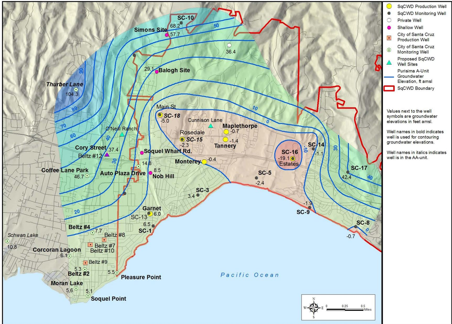
Figure 3-3 (2010): Groundwater Elevation Contours, Purisima A-Unit, Fall 2010
