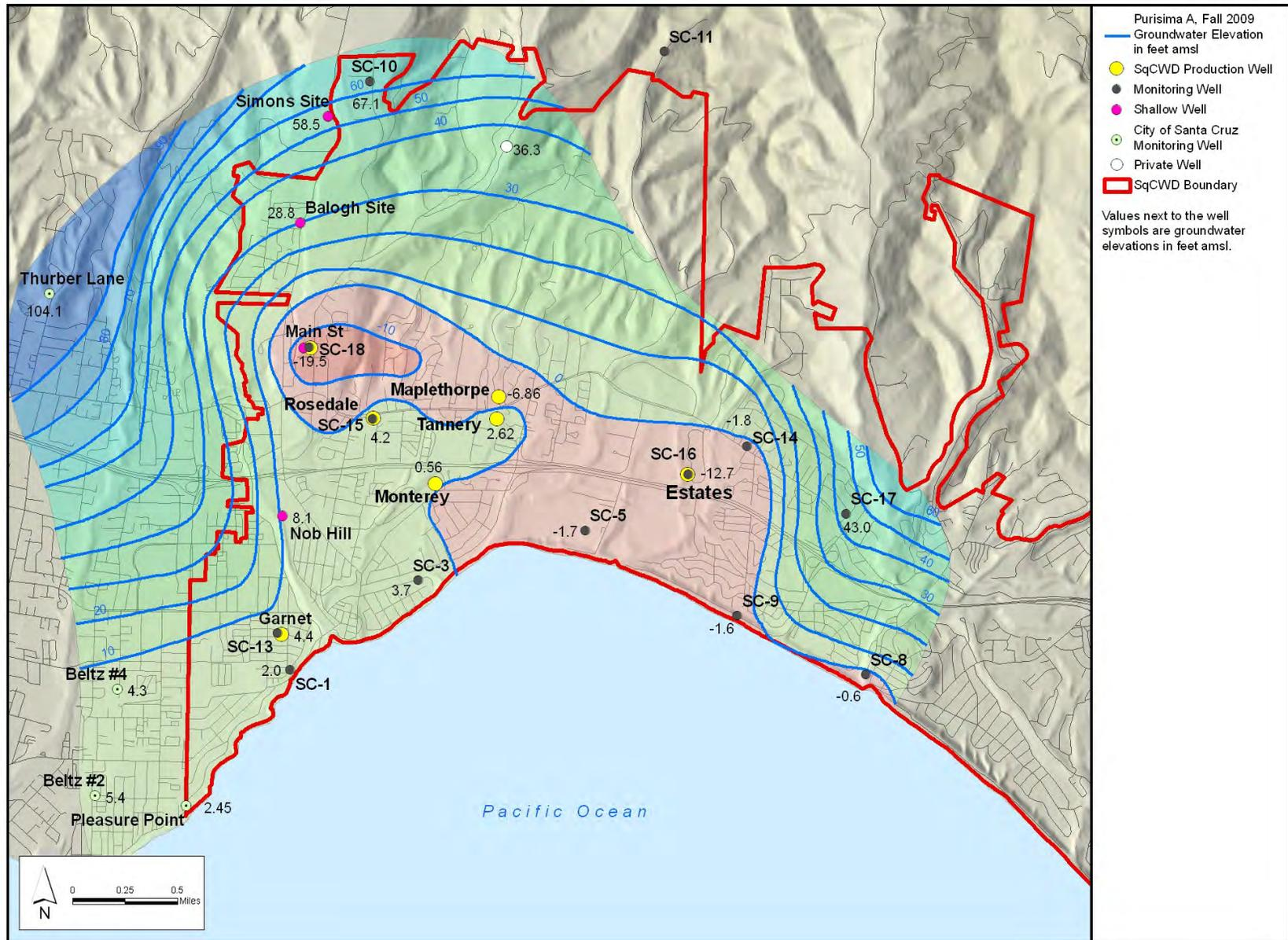
Figure 3-3 (2009): Groundwater Elevation Contours, Purisima A-Unit, Fall 2009
