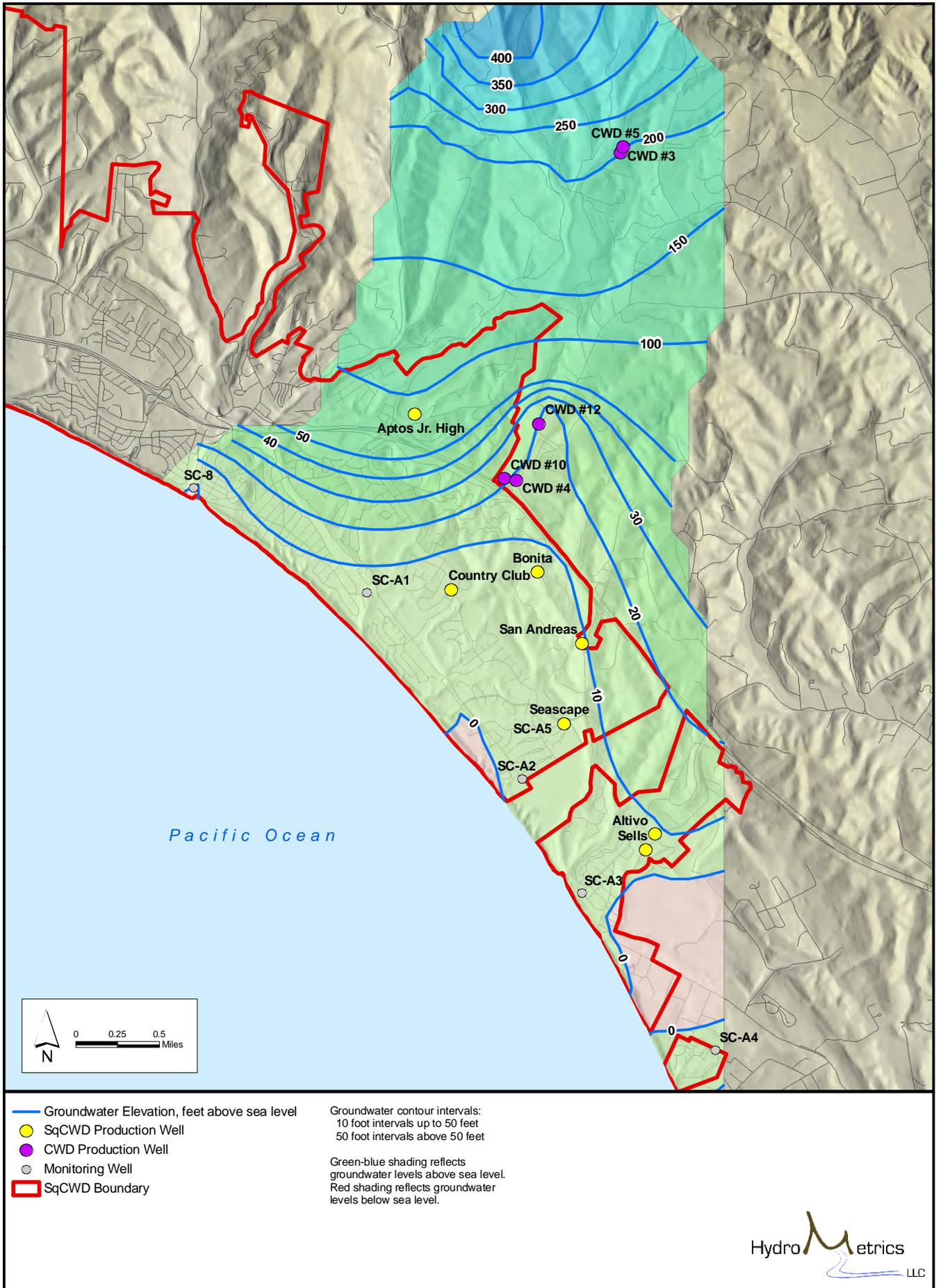
Figure 5-2 (2007): Groundwater Elevation Contours, Aromas Area, Spring 2007
