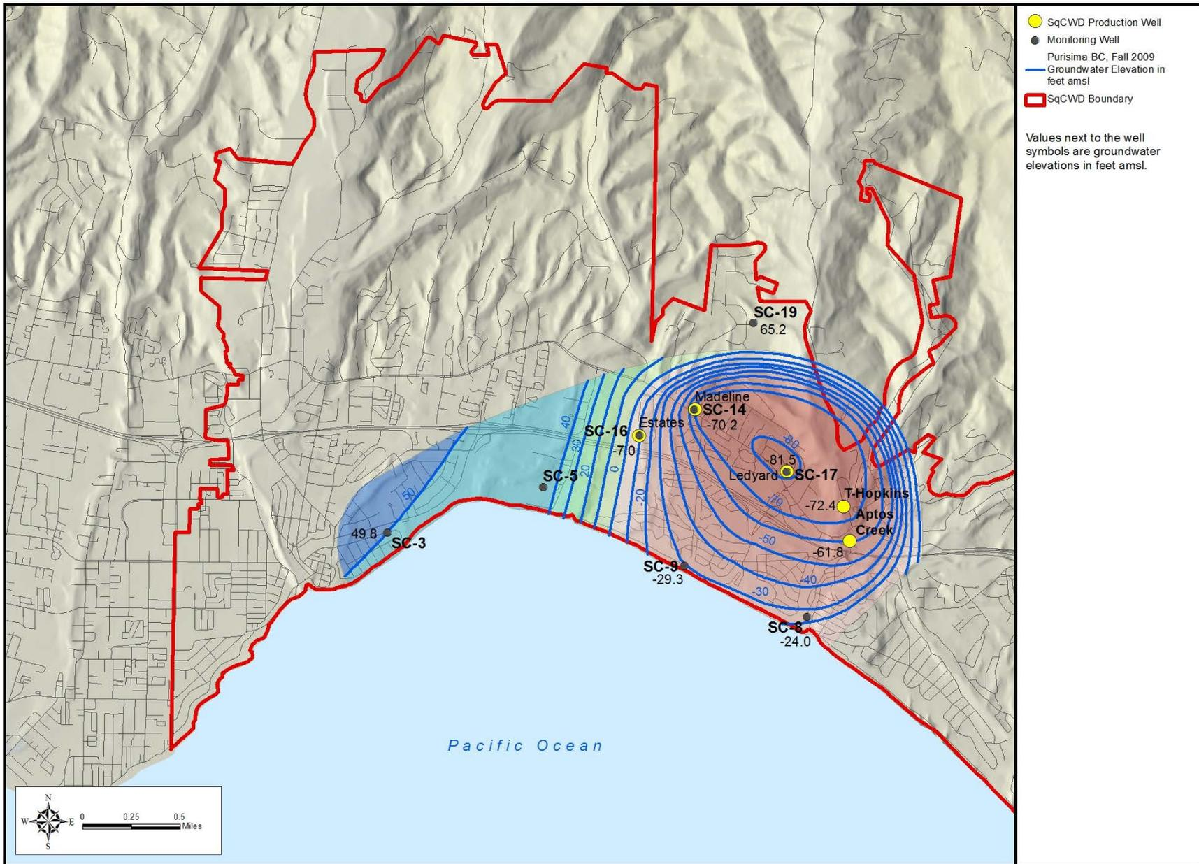
Figure 4-3 (2009): Groundwater Elevation Contours, Purisima BC-Unit, Fall 2009
