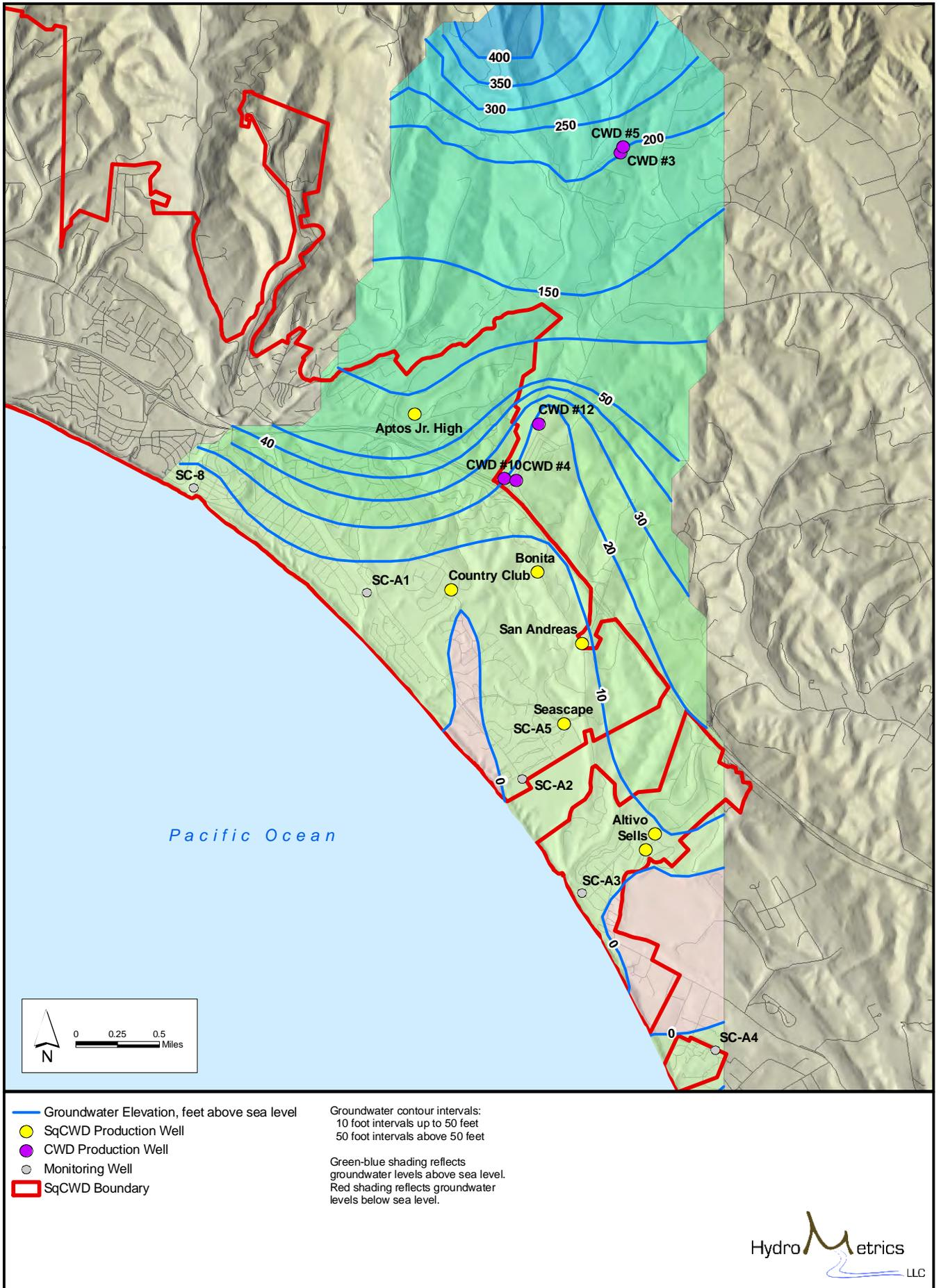
Figure 5-3 (2007): Groundwater Elevation Contours, Aromas Area, Fall 2007
