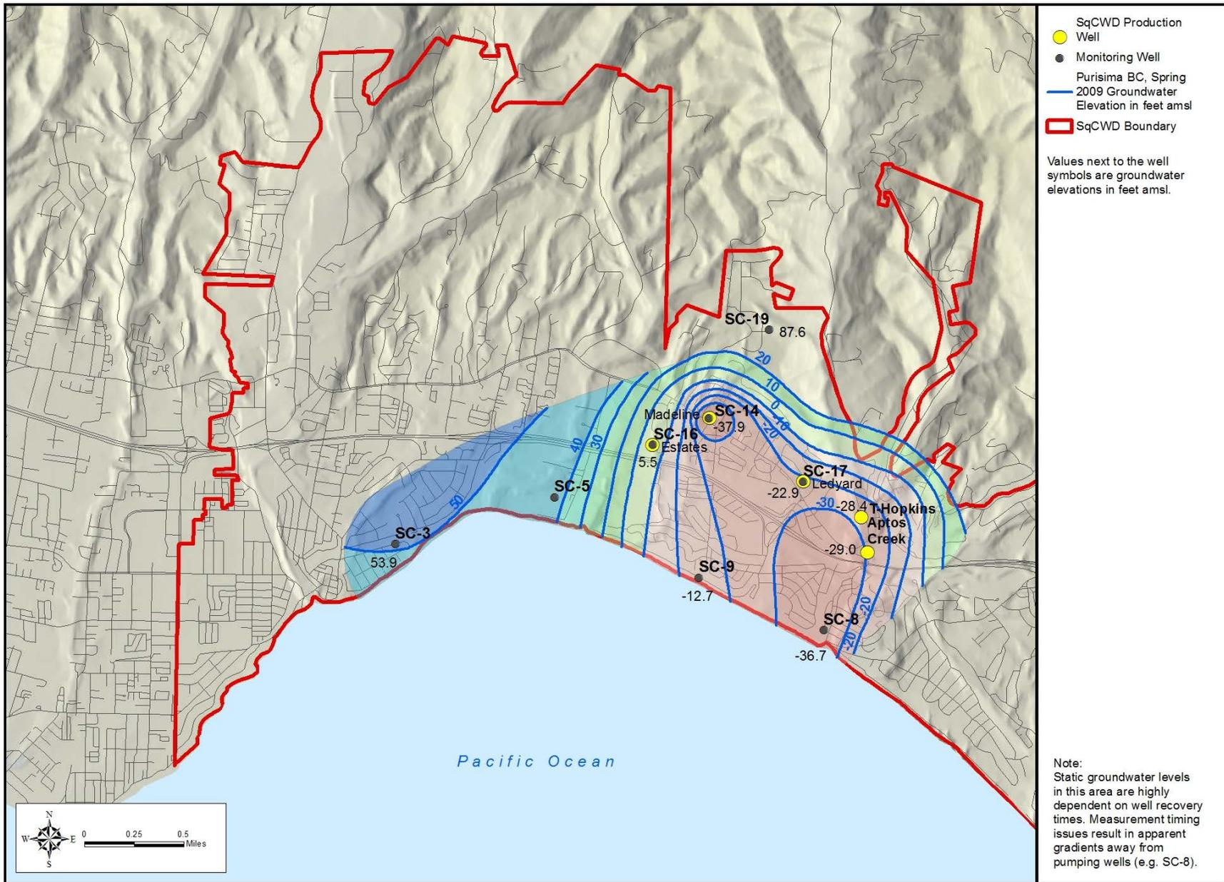
Figure 4-2 (2009): Groundwater Elevation Contours, Purisima BC-Unit, Spring 2009
