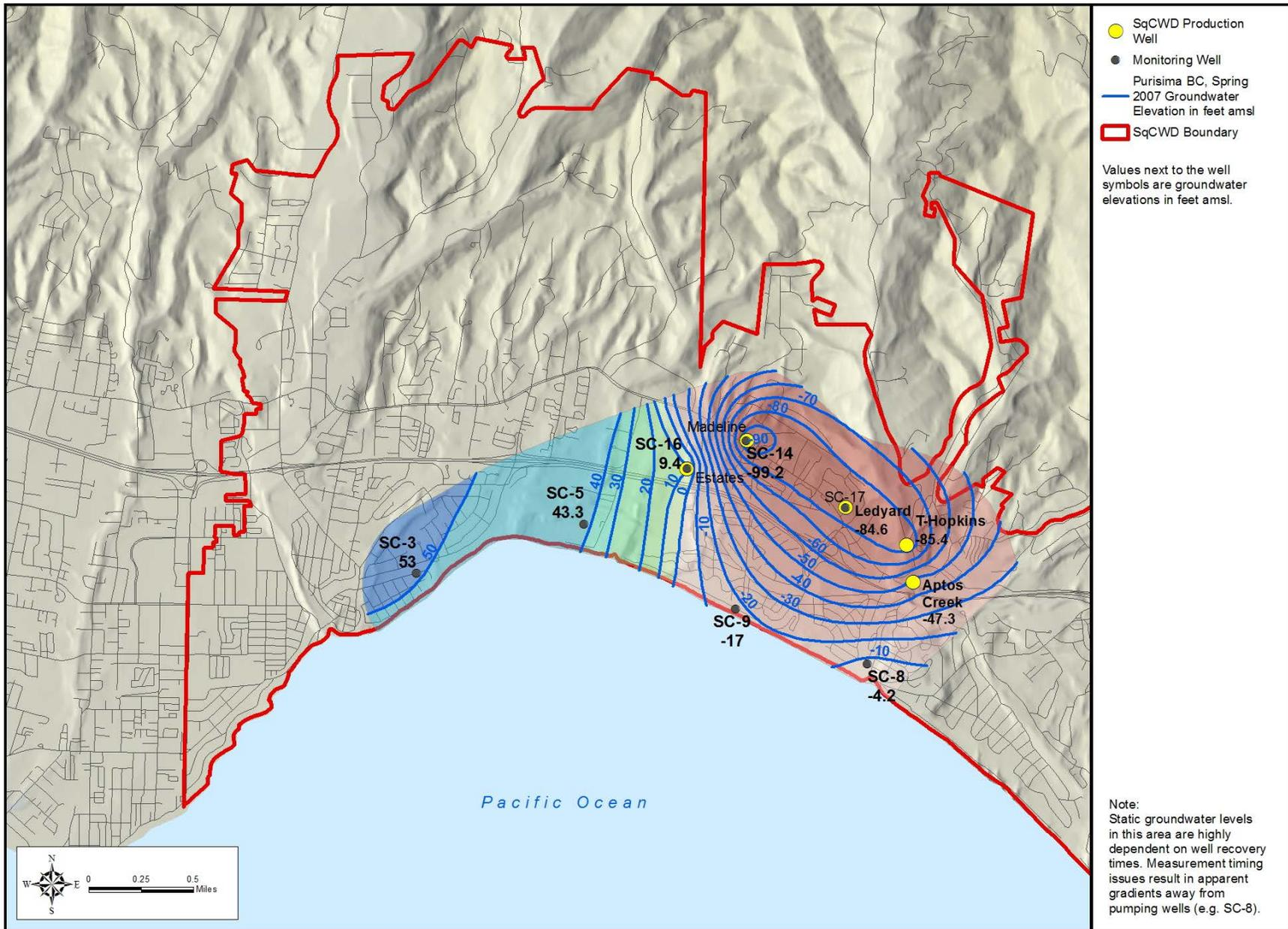
Figure 4-2 (2007): Groundwater Elevation Contours, Purisima BC-Unit, Spring 2007
