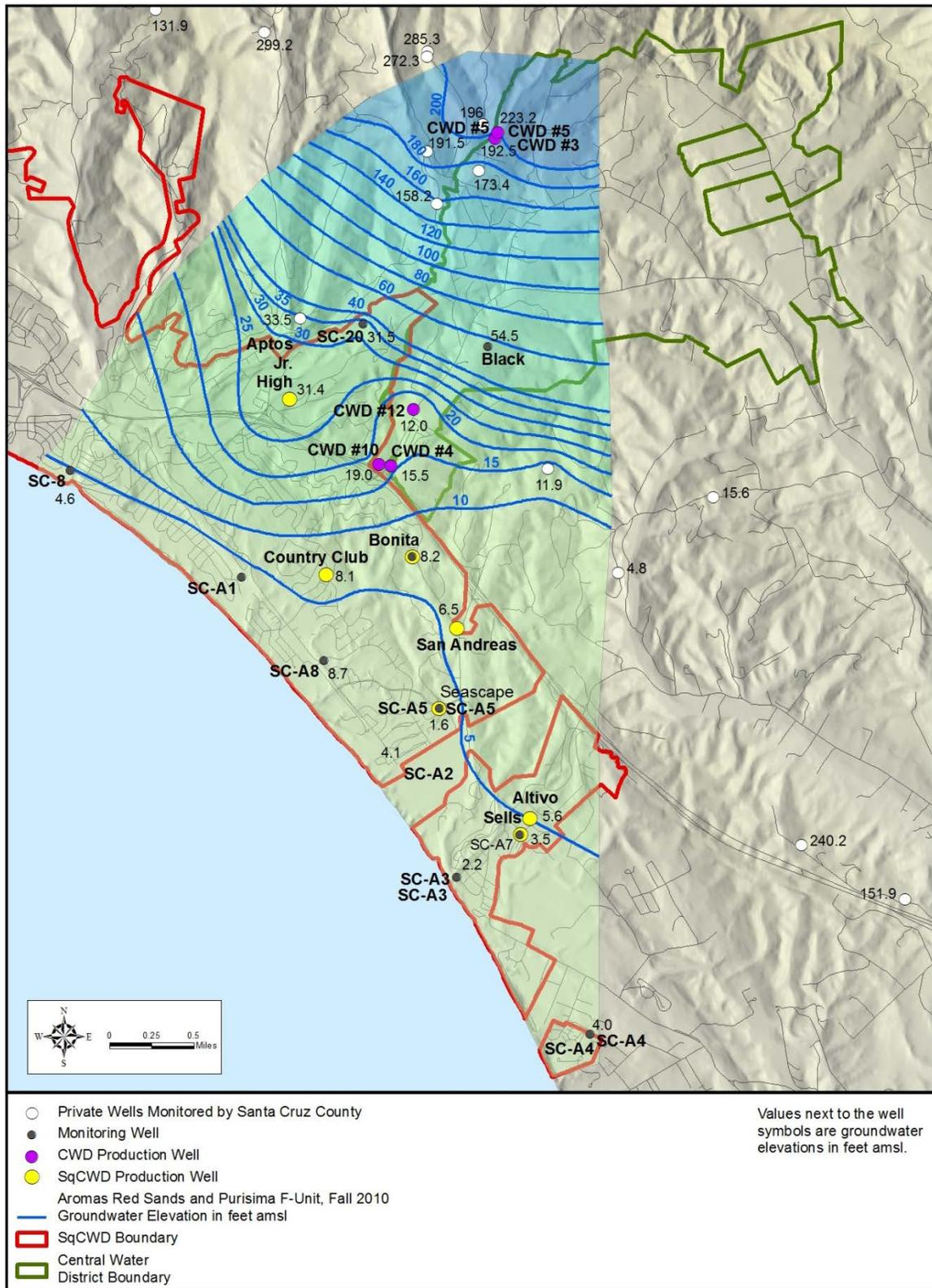
Figure 5-3 (2010): Groundwater Elevation Contours, Aromas Area, Fall 2010
