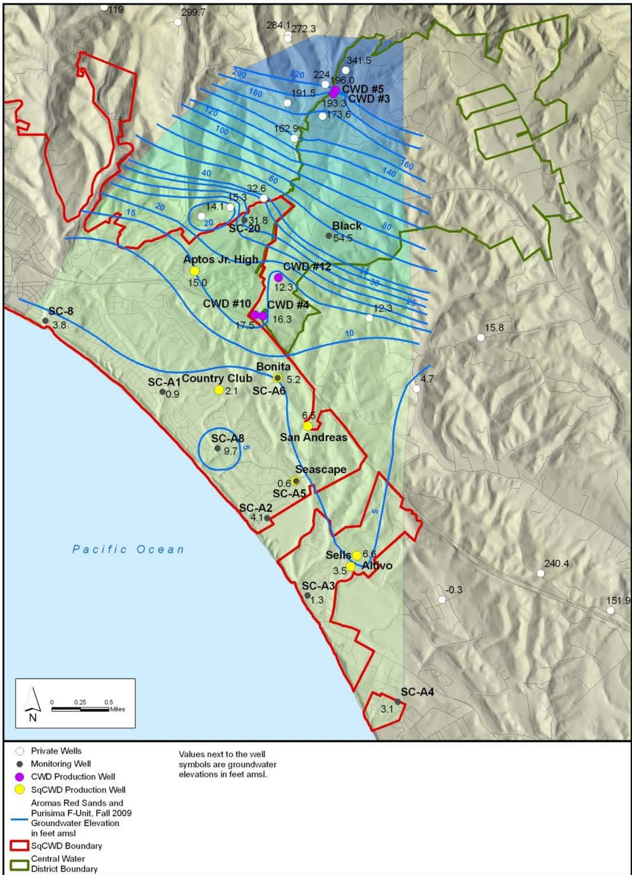
Figure 5-3 (2009): Groundwater Elevation Contours, Aromas Area, Fall 2009
