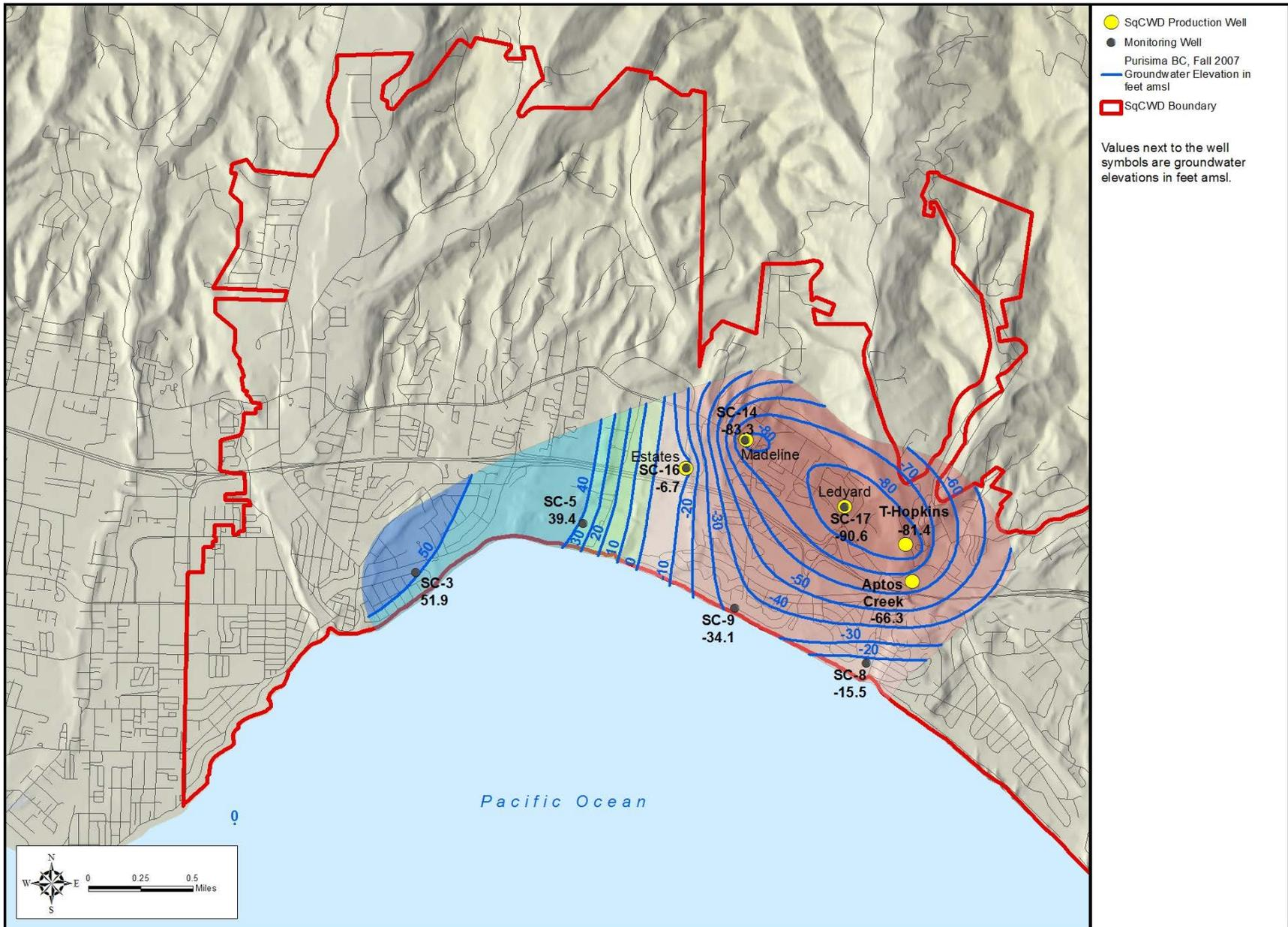
Figure 4-3 (2007): Groundwater Elevation Contours, Purisima BC-Unit, Fall 2007
