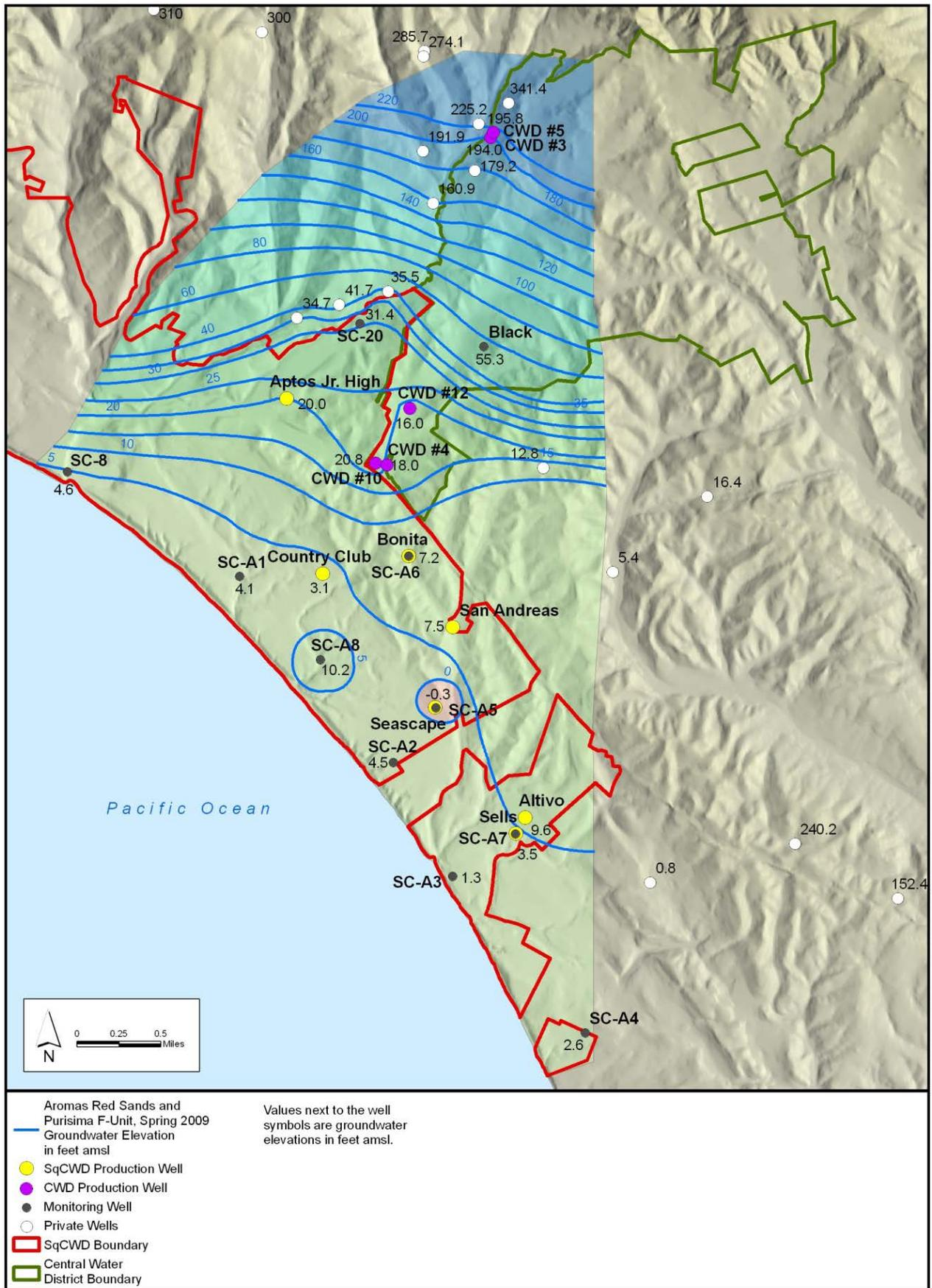
Figure 5-2 (2009): Groundwater Elevation Contours, Aromas Area, Spring 2009
