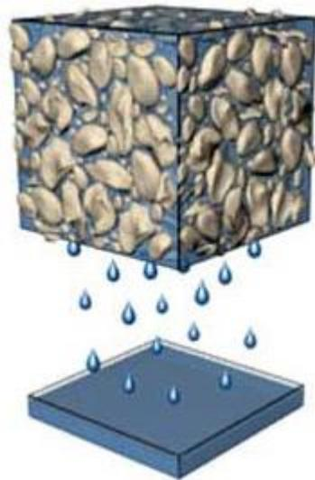
Drain 1 cubic foot of saturated sediments
