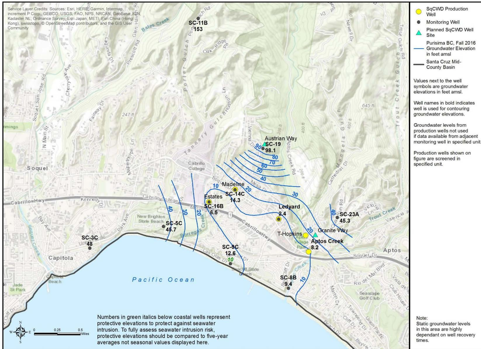
Figure 2-29. Groundwater Elevation Contours in Purisima BC-Unit, Fall 2016
