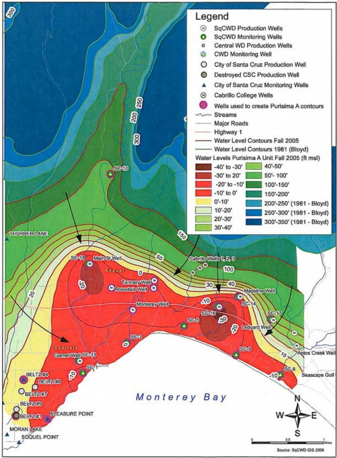
Figure 2-24. Groundwater Elevation Contours in Purisima A-Unit, Fall 2005
