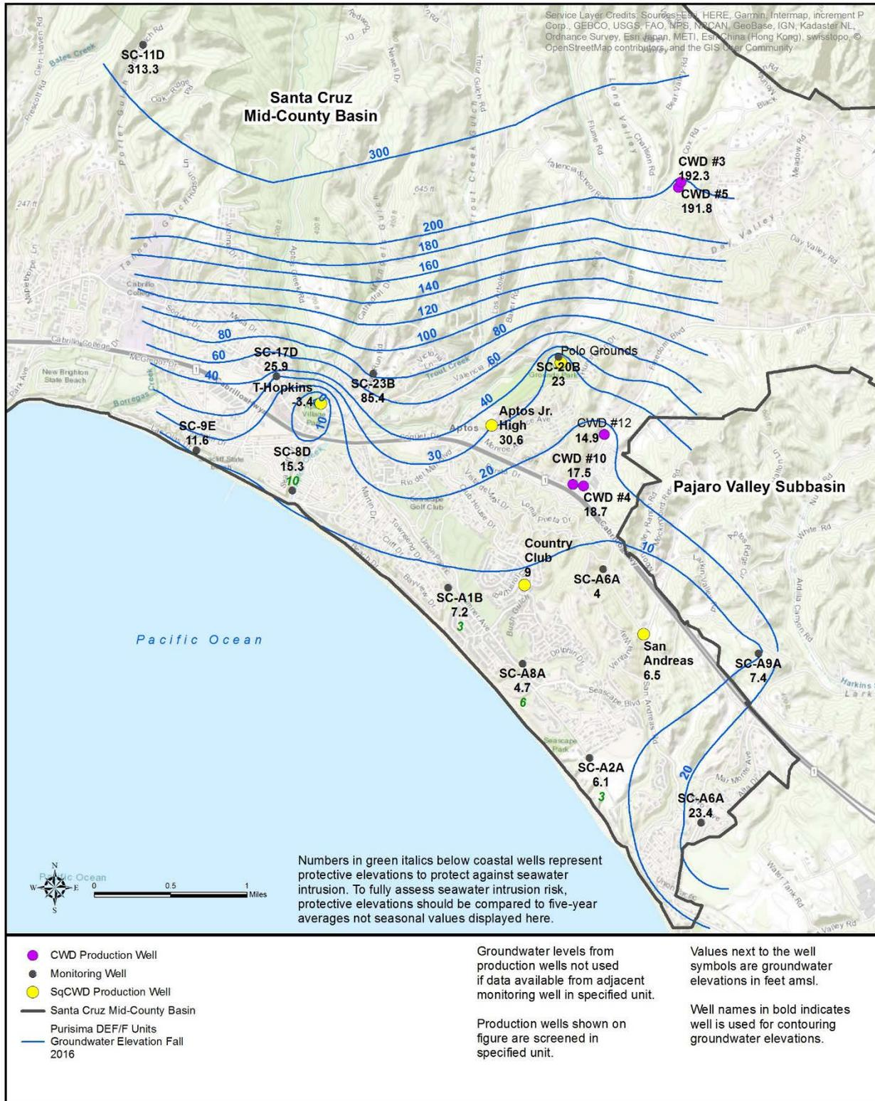
Figure 2-30. Groundwater Elevation Contours in Purisima DEF/F-Unit, Fall 2016
