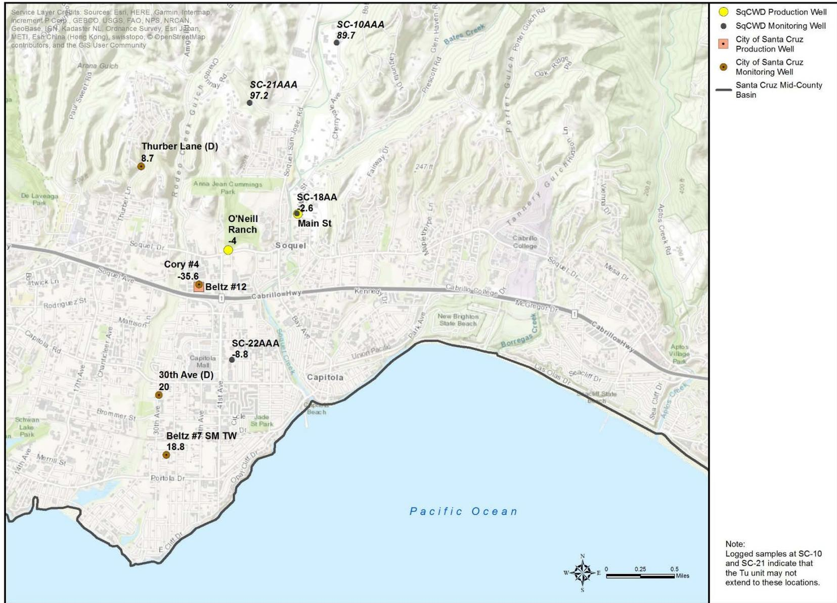
Figure 2-27. Groundwater Elevations in Tu-Unit, Fall 2016
