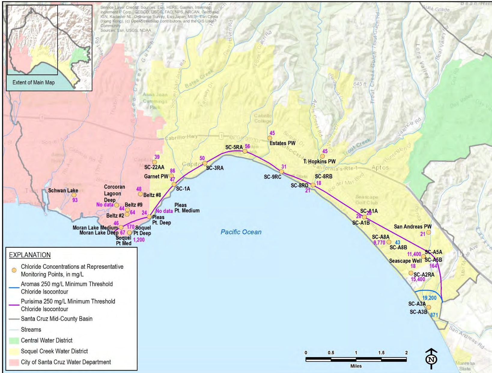
Figure 21. Water Year 2022 Maximum Chloride Concentration Map Compared to Minimum Threshold Isocontour
